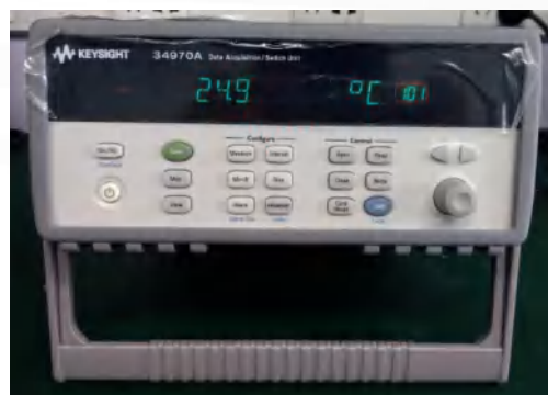
Verify the reliability test and test the surface temperature of the chip when it is working.
